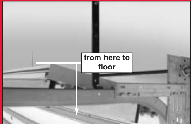
FIG. 2-1 Finding highest point of travel (sectional).
