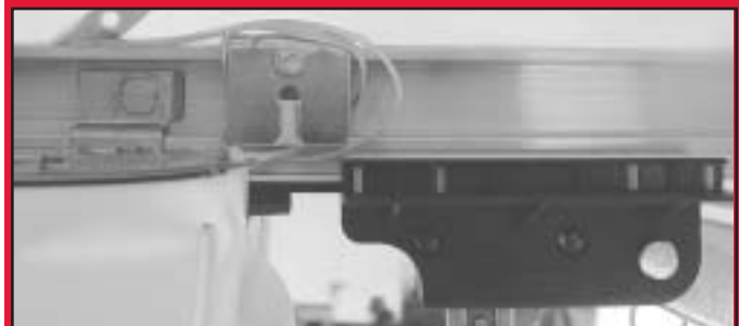
FIG. 7-4 Align “OPEN” limit switch.
