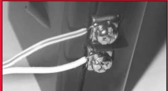
FIG. 3-7 Terminal attachments at STB.
