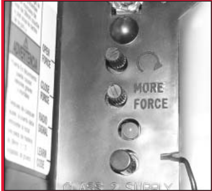
FIG. 7-1 Force adjustment screws.
