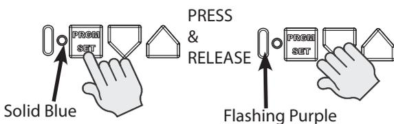
**NOTE:** The openers LEARN LED will time out in 30 seconds. Programming must be completed within 30 seconds.
