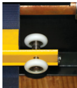
Articulating roller wind strut
